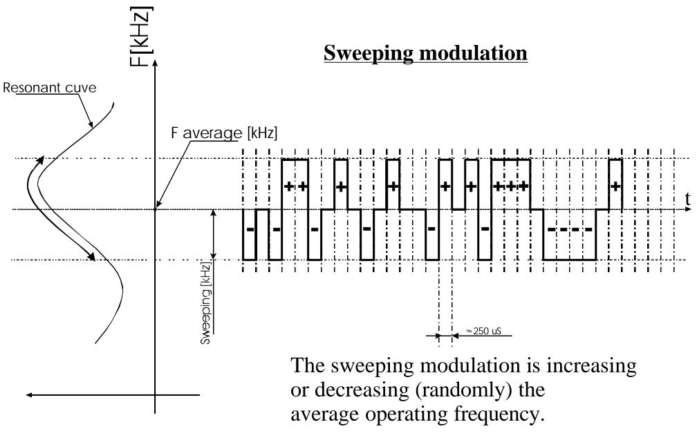
$F_{operating}[kHz] = F_{average}[kHz] + /- Sweeping[kHz]$
