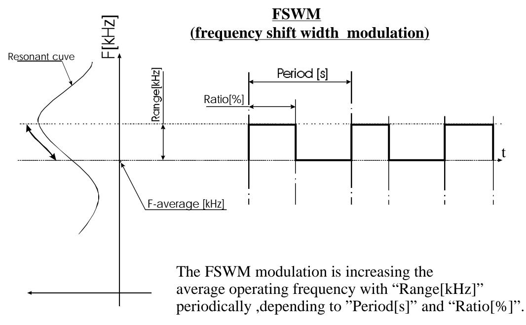
$F_{operating}[kHz] = F_{average}[kHz] + Range[kHz]$
