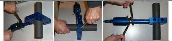
Pictures presenting ultrasonic converter with water jacket (upper part), wave-guide (middle part) and aluminum clamps on the reactor tube (bottom). Apply fastening of clamps, slowly, symmetrically and gradually (on both sides) until reaching **30 Nm torque** value (use proper torque wrench; -not presented on the pictures here). For fixation (screwing, unscrewing) of converter and wave-guide use here presented wrenches.
