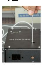
Increase the inductive compensation until find a maximum of current. The maximum current show the good resonance
