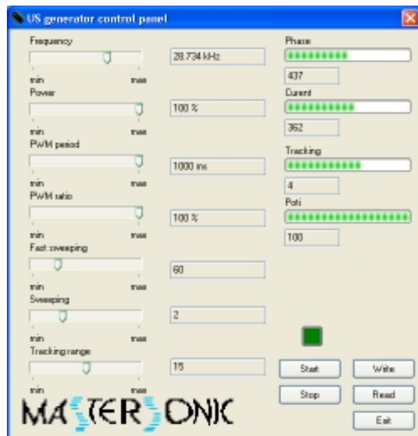
Figure 5. PC Windows Control Panel
