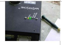
The yellow LED is ON the green LED blinking
