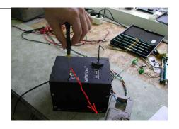
Turn the potentiometer (OV) on the right and find the good resonance
