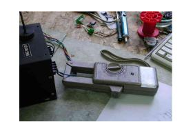
Conect Ampermeter clamp to power supply
