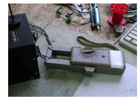
Conect Ampermeter clamp to power supply
