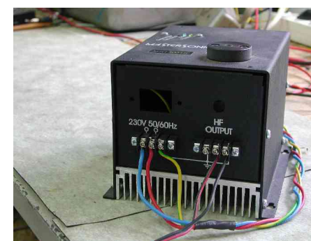
Conect Acoustic load to HF output terminals
