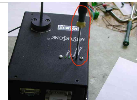
Turn the Potenetiometer (OV) on the left end
