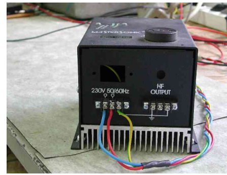
Conect power suply terminal
