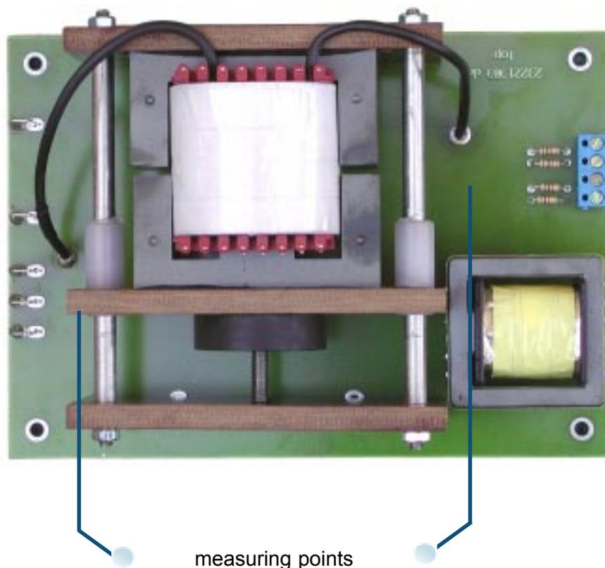
Fig. 7.1. Compensating Inductivity measuring
