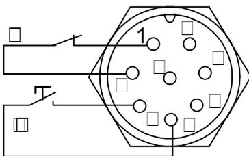
Fig. 9.2. External On/Off Power Control
