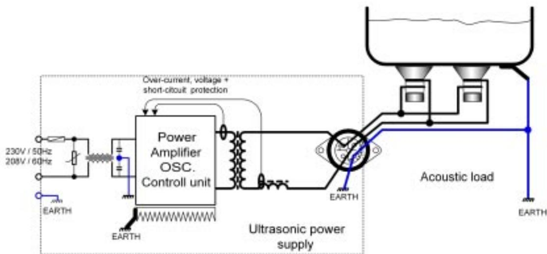
**Fig. 2.6. Recommended 3-wire Acoustic Load connection.**
