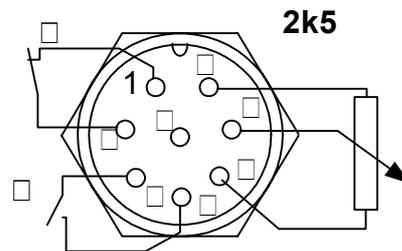
**Fig. 2.3. Connector for external ON/OFF Power Control**
