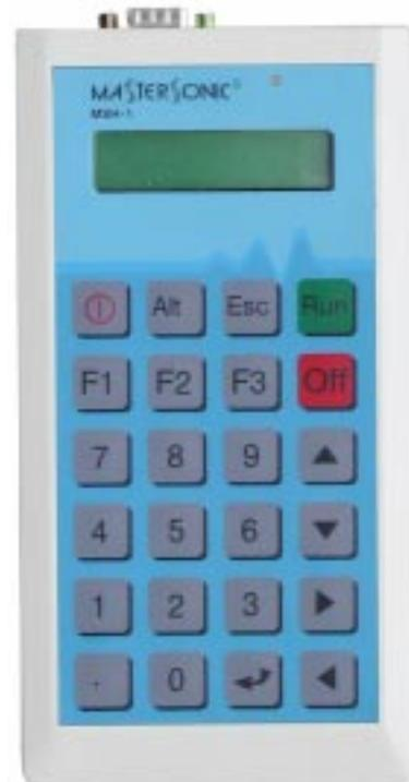
**Fig. 4.1. MSH-1 Remote Control Panel**
