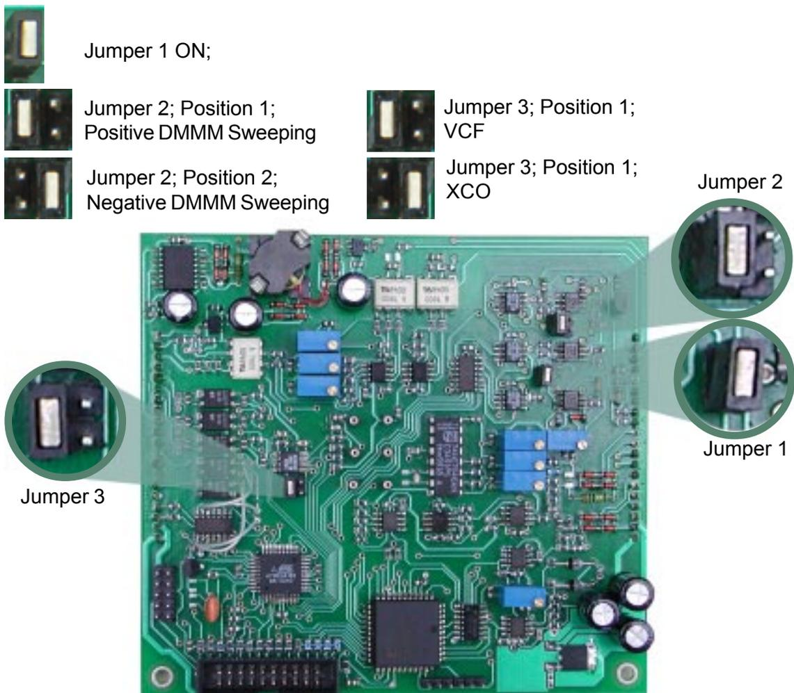
**Fig 9.1. Control Board Jumpers**
