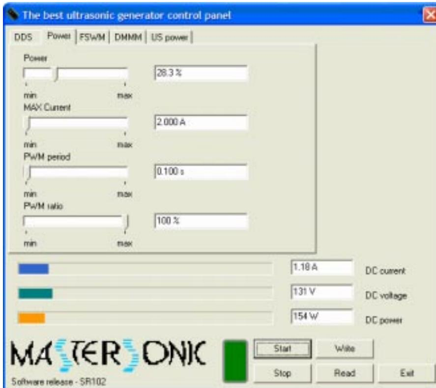
Fig. 6.3. MSG.x00.IX.yF software. Power Panel.
