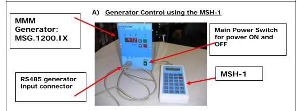
1. Plug-in the connectors between the Handheld Control Unit MSH-1 and RS485-connector on the front panel of the MSG.1200.IX generator. Handheld Control Unit MSH-1 will operate taking the power directly from the generator (no need for external DC power supply). See instructions regarding how to use MSH-1 in the system manual-:
