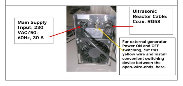
2. Connect the Ultrasonic System and Main Power Supply cable to the rear panel of the MGG.1200.IX generator. Attention: Apply European 230 VAC, 50/60 Hz, 30 Amp. input power line. When using step-up or step-down transformer, use a 5 kW transformer (to have large safety margin for pulsed-power operations). See instructions in the system manual:
