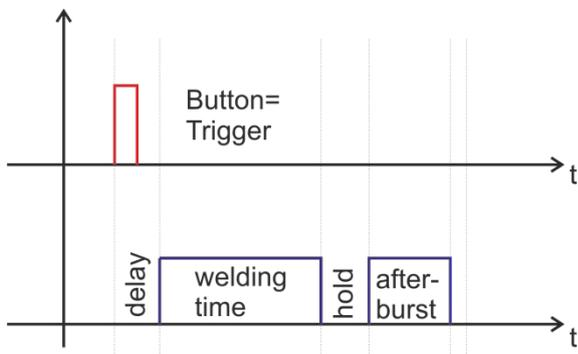
The generator allows **carrying** out the welding cycle by three criteria:
