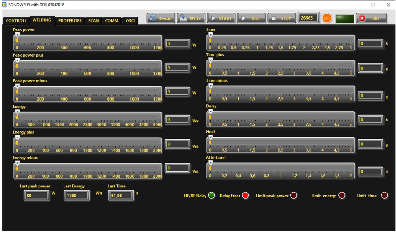
Before setting the welding regime you need to Select TRIGGER Mode for the button – you can do it in PROPERTIES Tab or from the Display.
