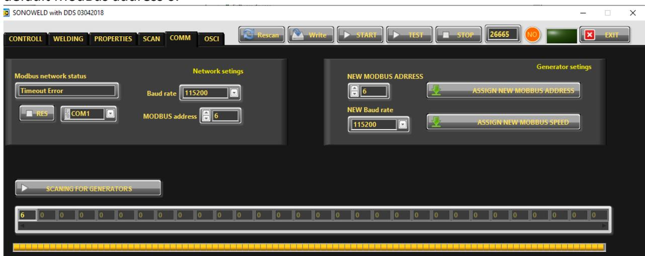
Press "SCANNING FOR GENERATORS". After scanning (the yellow bar will become full in a few seconds), you will find the address (es) of the available generator(s) you will drive. Check if the value of the address in "MODBUS address" field is correct and if needed change it with the value shown in the table below the button "SCANNING FOR GENERATORS". Beat counter will become alive and will
