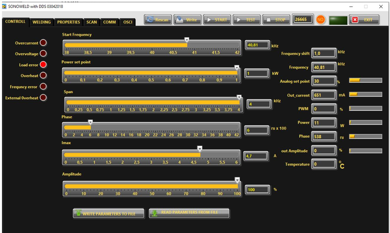
7. Go to CONTROLL Tab. The very first step is to press the button RESCAN to have all parameters and settings from the generator uploaded in Labview software.
