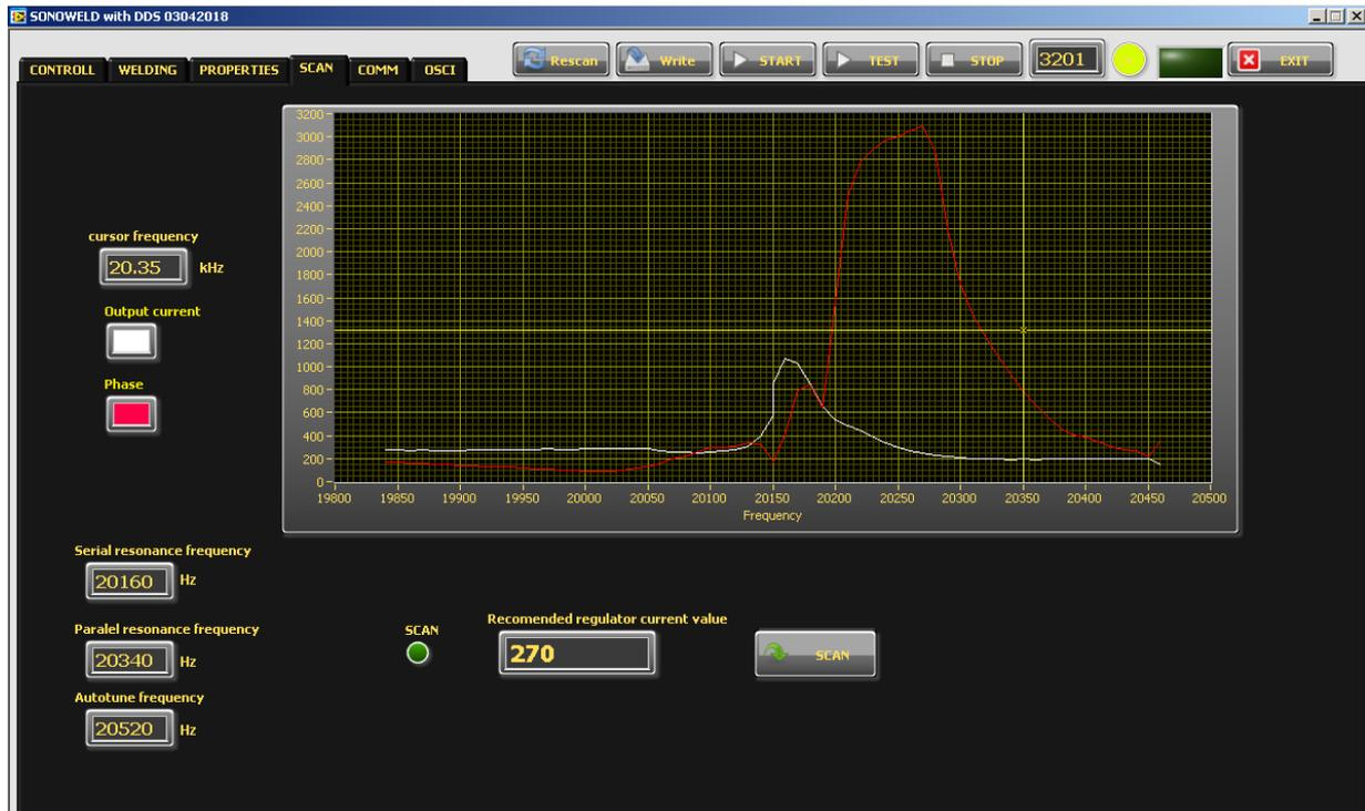
11. Press the SCAN button. The scanning procedure starts. There is a drawing consisting of phase characteristic (red line) and current characteristics (white line). It should be similar to the picture with well-defined phase feature. This diagram shows the actual operating parameters of the transducer. If necessary, pick new Fstart and SPAN (in CONTROL tab).
