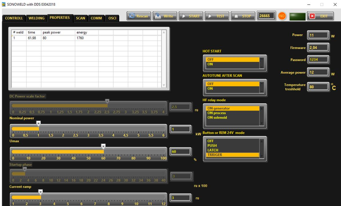
In PROPERTIES Tab you can select the HF Relay Mode(see right bottom corner) from three options:
