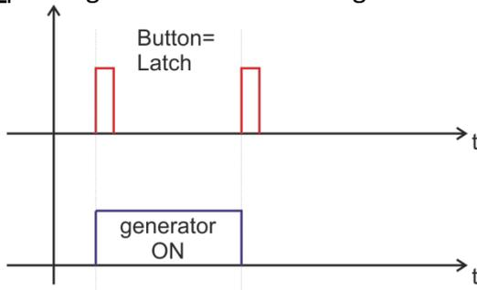
**TRIGGER** - pushing the button once the welding cycle starts.
