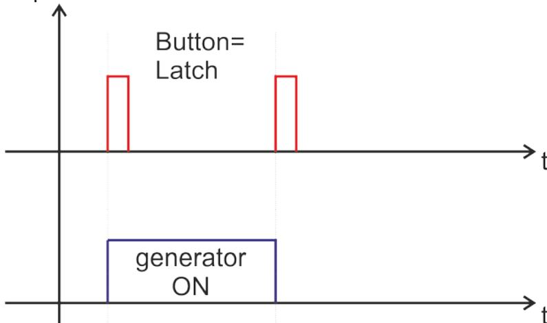
**TRIGGER** – pushing the button once the welding cycle starts.
