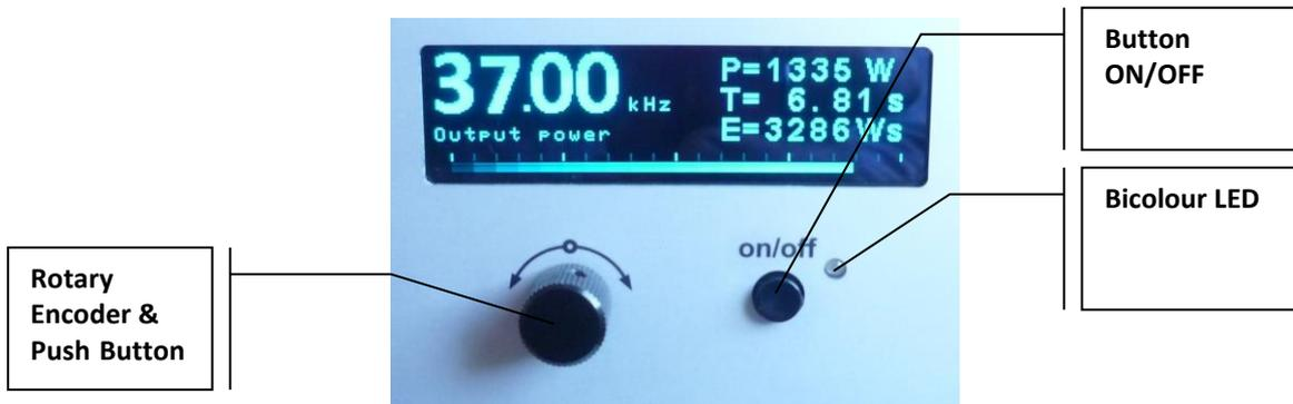
**Bicolour LED:** Lights up **green** when generator is switched on and works properly
