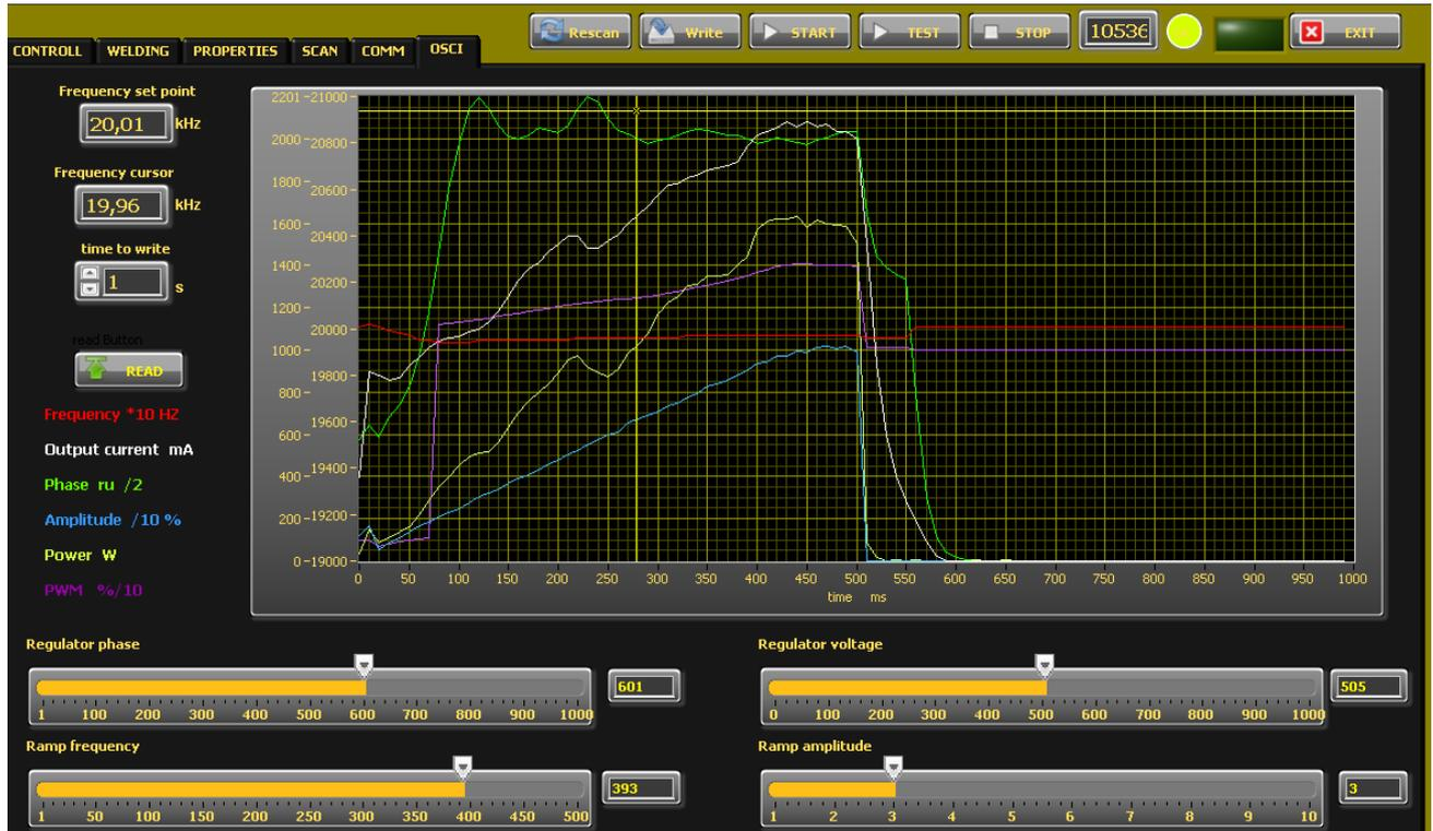
An oscilloscope allows us to follow the following parameters during welding cycle:
