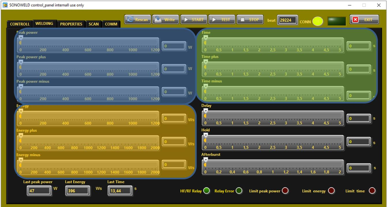
On this tab we can adjust the welding parameters such time, power and energy.
