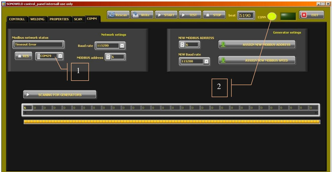
1. Select the exact COM port(1) to which the adapter is connected from the drop down menu.
