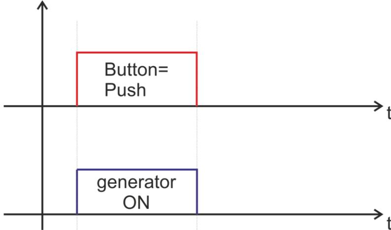
**LATCH** - pushing the button once the generator starts, pushing the button again the generator stops.
