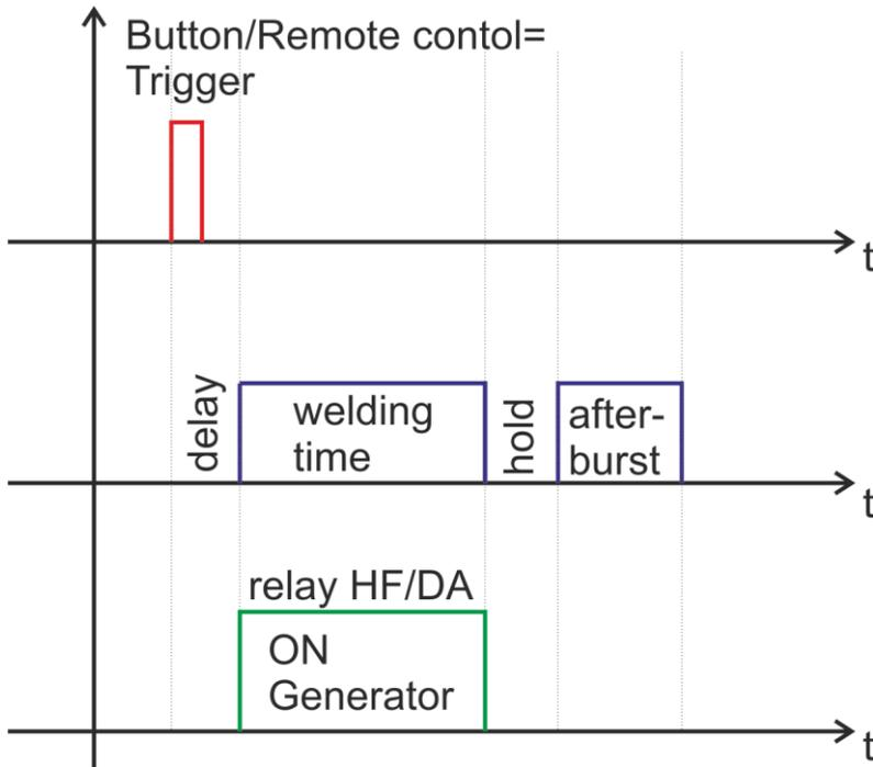
**ON process** – the relay is ON during whole process, including delay, welding time, hold and afterburst.
