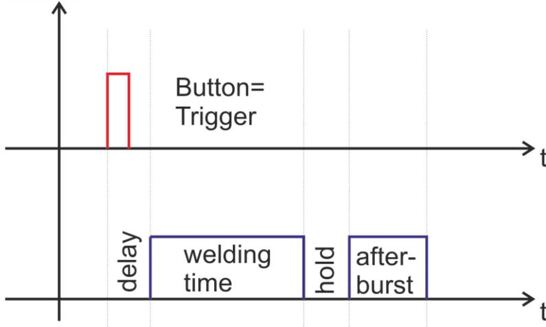
**If time, power or energy parameters are settled, Trigger mode must be selected.**
