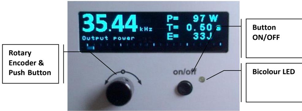
**Bicolour LED:** Lights up **green** when generator is switched on and works properly
