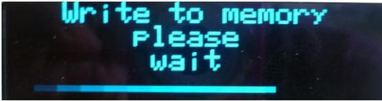
This window appears when you PRESS AND HOLD the Rotary Encoder for 2 sec.
