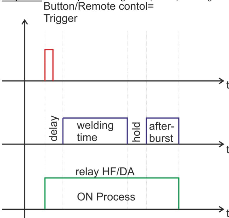
**ON solenoid** - the relay is ON during delay, welding time and hold.
