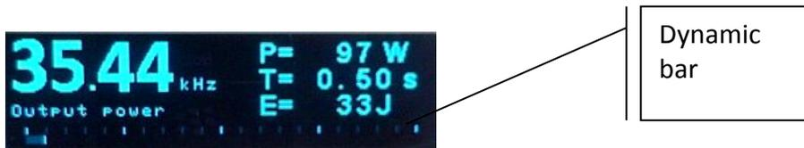
After the generator is powered on, the initial screen contains the following status information.
