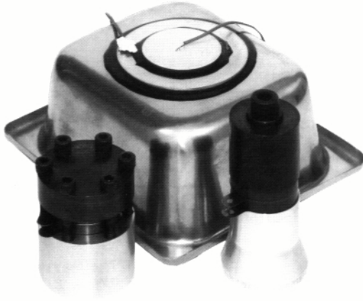
Fig.6.5 Some high-intensity ultrasonic transducers for cleaning applications (see also Figs.6.8, 6.9 and 6.10)
