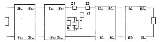
Fig. 4. The equivalent circuit of a transducer-horn system.
