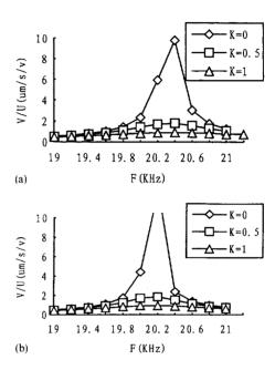
Fig. 6. Voltage transforming coefficients of a transducer-horn system vs. frequencies and loads; (a) area ratio of horn 1:1, (b) area ratio of horn 4:25.
