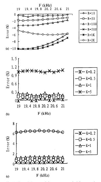
Fig. 19. Theoretical errors of the wattmeter method for measuring output acoustical power under different loads and frequencies; (a) clamped transducer system, (b) transducer-horn system (1:1), (c) transducer-horn system (4:25).
