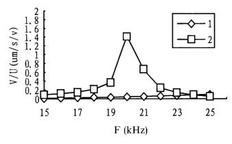
Fig. 15. Voltage transforming coefficients of the transducer vs. frequencies; (1) in a clamped transducer system driven with the same electrical generator at the same time, (2) single transducer.
