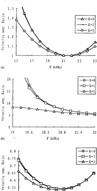
Fig. 2. The velocity amplitude ratios of front and back end face of the transformer vs. frequencies and loads; (a) area ratio 1:1, (b) area ratio 4:25, (c) area ratio 25:9.
