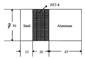
Fig. 5. The dimensions of the transducer.
