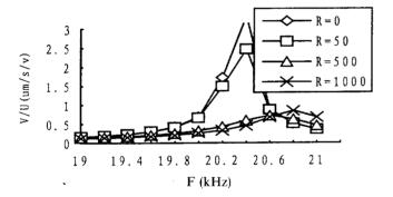
Fig. 12. Voltage transforming coefficients of the driven transducer in a clamped transducer system vs. loads and frequencies.
