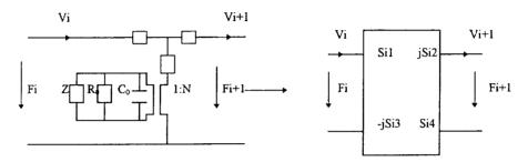
Fig. 11. Simplified equivalent circuit and matrix of ceramics groups connected with Z.
