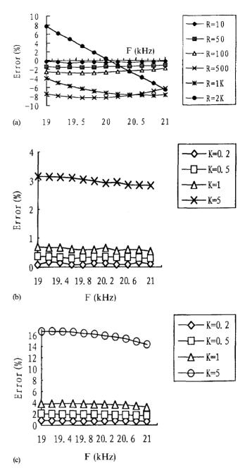
Fig. 18. Theoretical errors of the wattmeter method for measuring ouput acoustical power under different loads and frequencies without considering the dielectric losses; (a) clamped transducer system, (b) transducer—horn system (1:1), (c) transducer—horn system (4:25).
