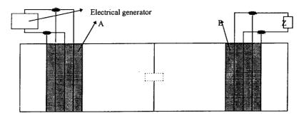
Fig. 10. Clamped transducer system.
