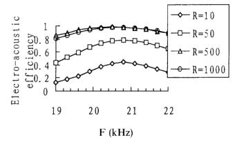
Fig. 14. Efficiencies of a clamped transducer system vs. frequencies and loads.
