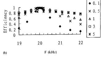
Fig. 7. Efficiencies of transducer-horn system vs. frequencies and loads; (a) area ratio of horn 1:1, (b) area ratio of horn 4:25.
