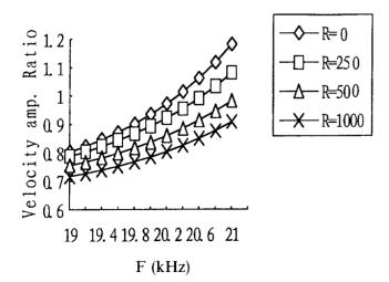
Fig. 13. Velocity amplitude ratios of front and back end face of the driven transducer in a clamped transducer system vs. loads and frequencies.
