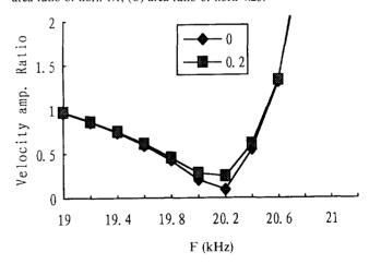
Fig. 9. Velocity amplitude ratios of a position (near node) and back end face of the transducer in a transducer-horn system (4:25) vs. frequencies and loads.
