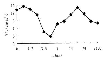
Fig. 17. Variation of voltage transforming coefficients of the driven transducer in a clamped transducer system at resonance frequency with inductance L. One transducer was driven, the other was connected with inductance L.
