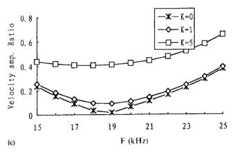
Fig. 3. Velocity amplitude ratios of a position (near node) and back end face of the transformer vs. frequencies and loads; (a) area ratio 1:1, (b) area ratio 4:25, (c) area ratio 25:9.
