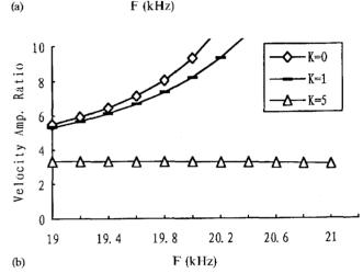
Fig. 8. Velocity amplitude ratios of front and back end face of the transducer in a transducer-horn system vs. frequencies and loads; (a) area ratio of horn 1:1, (b) area ratio of horn 4:25.
