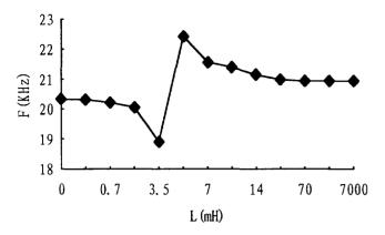
Fig. 16. Variation of the resonance frequency of a clamped transducer system with inductance L. One transducer was driven, the other was connected with inductance L.
