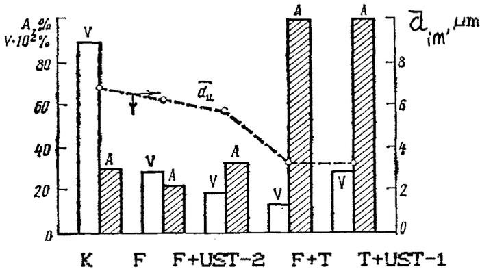
Figure 4. Effect of fine filtration (Usfirls-process) using multilayer screen filters (F) combined with other kinds of molten metal treatments on structure of 1973 (0.3% Zr) ingots, 270 mm in diameter (see explanations in text).
