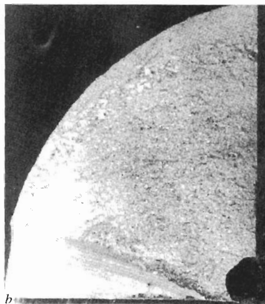
Figure 10.12. Fracture of grade Cr18Ni15B3 boron steel ( \times 8 magnification): (a) control ingot, (b) ultrasonically solidified ingot.
