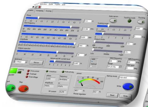
**Ultrasonic Generator Control Panel**
