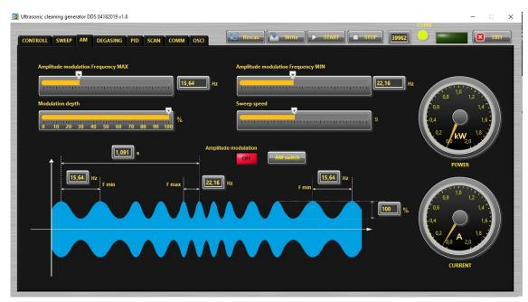
**Amplitude modulation frequency MAX –** This the maximum value of the frequency of the amplitude modulation.
