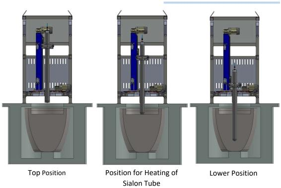
7.2 DIMENSIONS OF WORK – Minimum and Maximum Sialon Tube Positions
