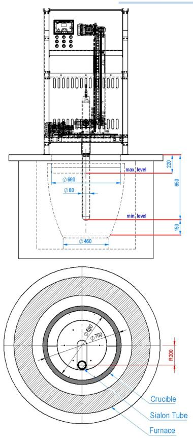
**NOTE:** The Distance from center of Sialon Tube to center of the crucible can range from R = 0 mm to R = 220 mm (R = 0 mm must be used with AUTOMATIC Mode – Center Cycle).
