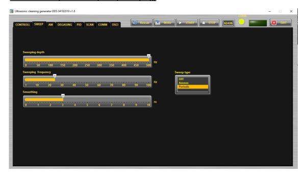
**Sweeping depth**– This is the deviation of the sweeping frequency around the central operation frequency in Hz.
