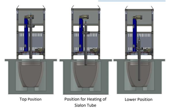
7.2 DIMENSIONS OF WORK – Minimum and Maximum Sialon Tube Positions
