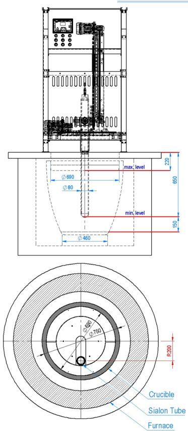
**NOTE:** The Distance from center of Sialon Tube to center of the crucible can range from R = 0 mm to R = 220 mm (R = 0 mm must be used with AUTOMATIC Mode – Center Cycle).
