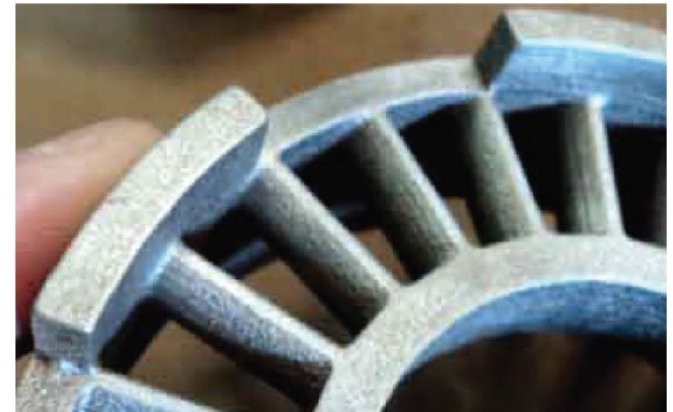
Additive technology Wear after 600 hours.
