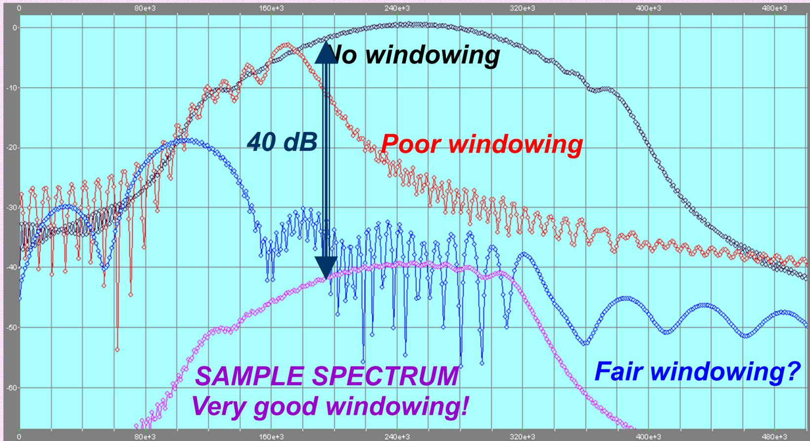
**Adequate WINDOWING is crucial in spectral analysis**
