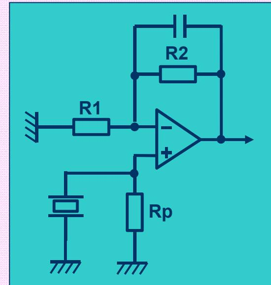
In a non-inverting voltage preamplifier, the equivalent input noise voltage spectral density is determined as follows ( $R1 \ll Req$ ):
