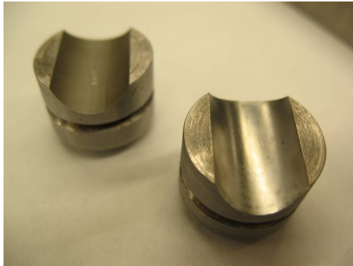
Figure 14: Preliminary results of 3D cavities (part in background was wire EDM cut, (part forfront) was \mu polished with polymer tool
