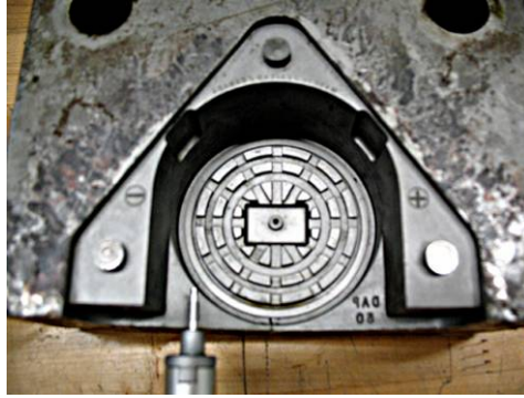
Figure 3: P20 mold cavity of truck alarm casing
