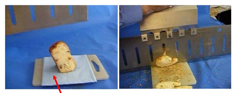
First cut realized without vibrations Next cuts: Ultrasonic Cutting
