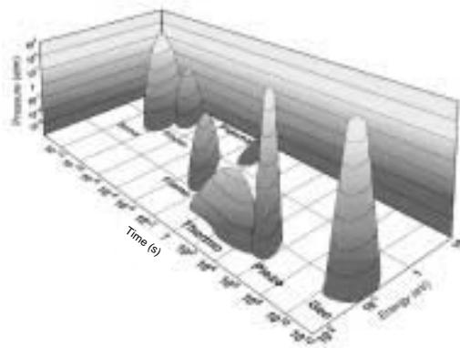
Sonochemistry consists of high-energy reactions under high pressures and short times.
