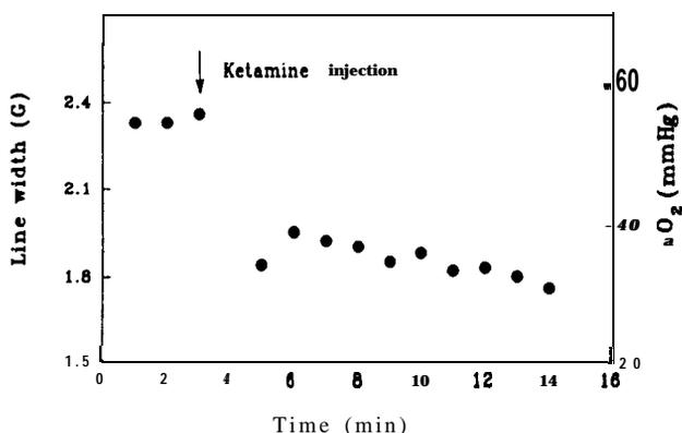
FIGURE 4 Effect of anesthetic on the  $[O_2]$  within a mouse. EPR spectra were recorded from the lower half of the body of the animal. The temperature of the mouse was maintained at  $37 \pm 2^\circ C$  with an infrared lamp. The microspheres were filled with 5 mM 7-DS in hexane.
