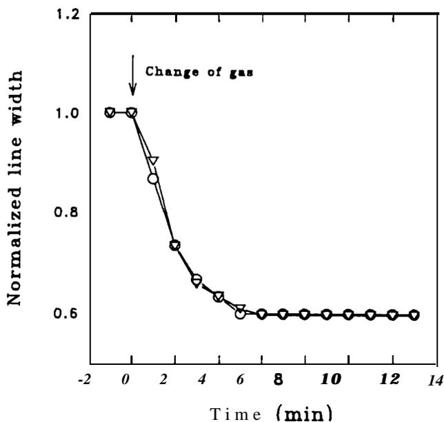
FIGURE 1 Kinetics of oxygenation inside and outside the microspheres. An aqueous solution containing  $^{15}\text{N}$ -PDT and microspheres filled with 7-DS in cyclohexane was drawn into a gas-permeable teflon tubing that was inserted in the quartz EPR tube. The perfusing gas was changed from nitrogen to air. The EPR line widths of "N-PDT ( $\circ$ ) and 7-DS ( $\nabla$ ) were measured simultaneously every 60 s.
