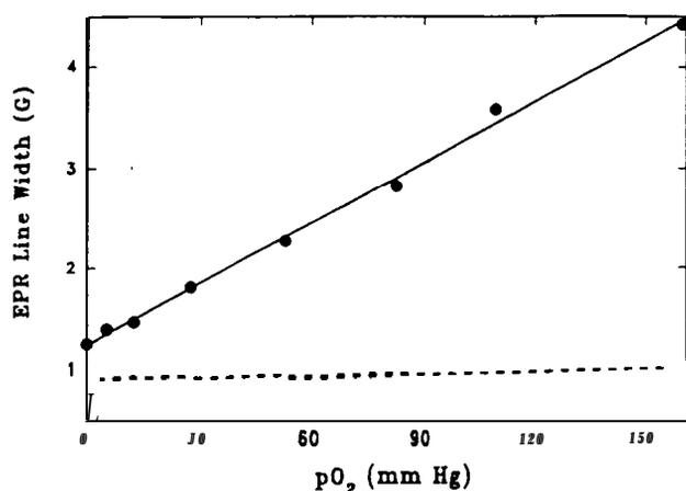
FIGURE 3 Calibration with  $[O_2]$  of the microspheres filled with 1 mM 16-DS in toluene. As a comparison, the dashed line shows the calibration of 16-DS in water. The line width of the central hyperfine line was used in these and all other figures.
