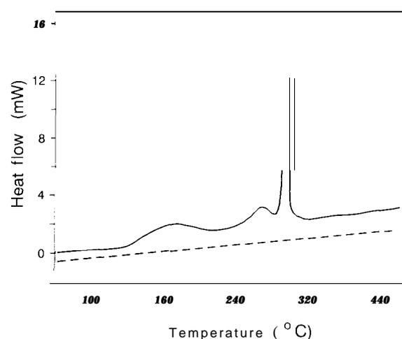
FIG. 2 Differential scanning calorimetry of amorphous (solid line) and crystalline (dashed line) iron powders, obtained at  $10^\circ\text{C min}^{-1}$  on a DuPont 1090 calorimeter.
