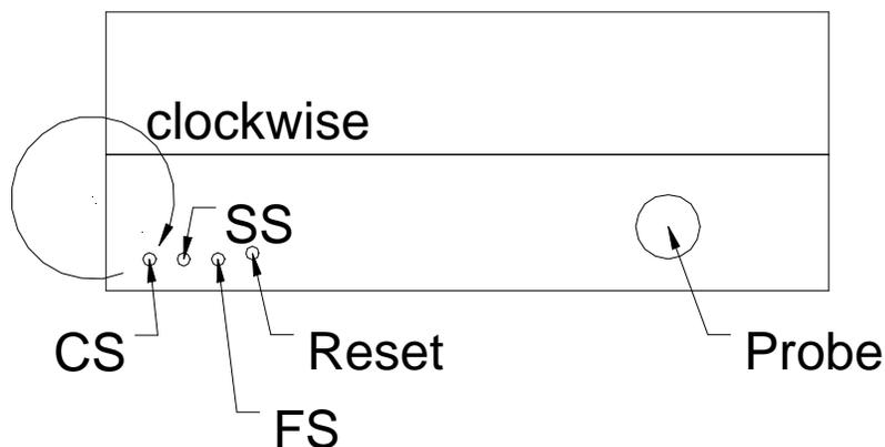
Ultrasonic cavitation energy meters have a **calibration screw (CS)** located on the top of the meter behind the receptacle for the ultrasonic probe. The location of the screw is shown on the drawing on the previous page. The **SS** and **FS** screws are disabled on the pb-500 meter. The procedure to calibrate the energy with this adjustment is as follows:
