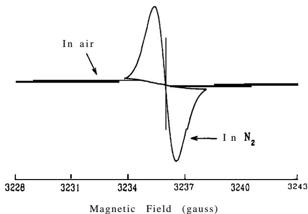
FIGURE 2 EPR spectra of microspheres filled with 2 mM 3-maleimido-proxyl in hexane equilibrated with  $\text{N}_2$  and air. The corresponding line width, which is used to calculate  $[\text{O}_2]$ , changed from 1.16 to 4.96 Gauss. This change is 60 times larger than the change in aqueous solution for this nitroxide.
