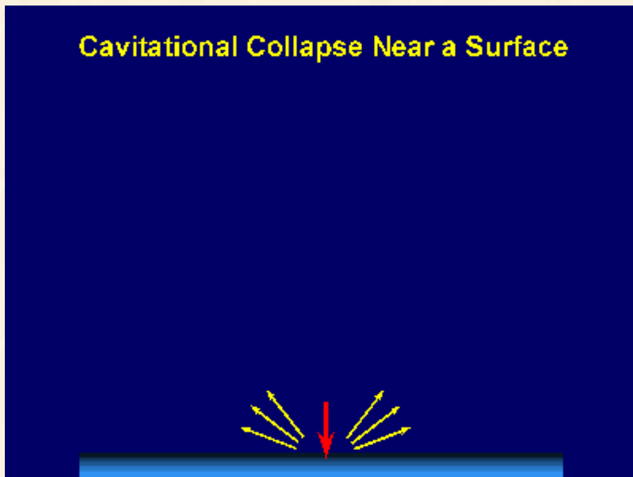
Fig. 7. Bubble collapse near an extended surface is distorted and leads to a shaped-charge effect with liquid jet impacts at >100\text{m/s} .
