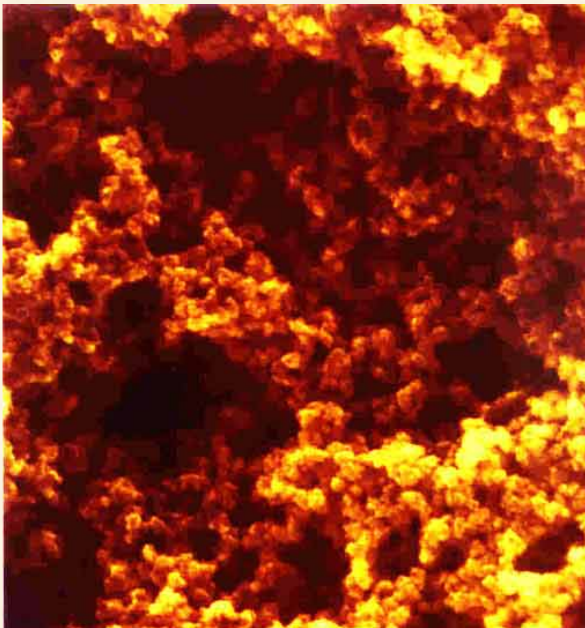
Fig. 5. Scanning electron micrograph of amorphous nanostructured iron powder produced from the ultrasonic irradiation of \text{Fe}(\text{CO})_5 . Particles making up this porous agglomerate are 10 to 20 nm in diameter.
