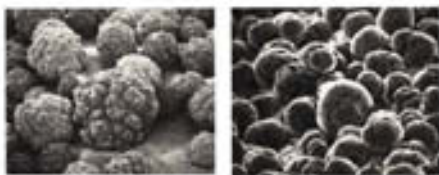
METAL SURFACES can be physically altered by ultrasound. Before this sample of nickel powder was irradiated with ultrasound (left) it had an unreactive crystalline coating on its surface. After irradiation (right) the coating was gone, exposing the nickel and boosting its reactivity. Without the coating the nickel powder becomes an excellent catalyst for chemical reactions. The magnification is about 100 diameters.
