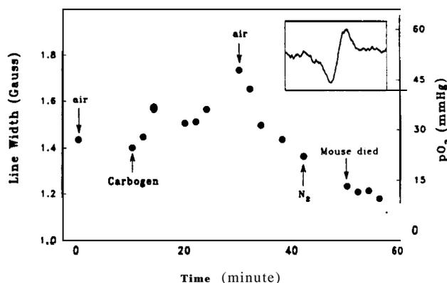
FIGURE 6 The change of  $[O_2]$  in the skeletal muscle of a mouse upon the variation of  $O_2$  content in the respiration gas. 100  $\mu l$  of microspheres of 5 mM 16-DS in cyclohexane were injected. The inset shows a typical spectrum of the middle line of the nitrogen hyperfine line. The animal died shortly after breathing  $N_2$ . Carbogen: 95%  $O_2$ , with 5%  $CO_2$ .
