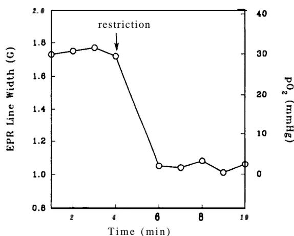
FIGURE 5  $[O_2]$  in the skeletal muscle of a mouse with and without constriction of blood flow. The constriction was achieved by means of a ligature around the upper leg. The response to decreases of  $[O_2]$  was indicated by a narrowed line width and increased line height. The microspheres were filled with 5 mM 10-DS in cyclohexane.
