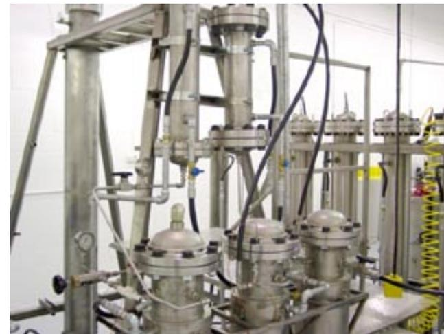
Pilot Plant Supercritical Fluid Extractor
