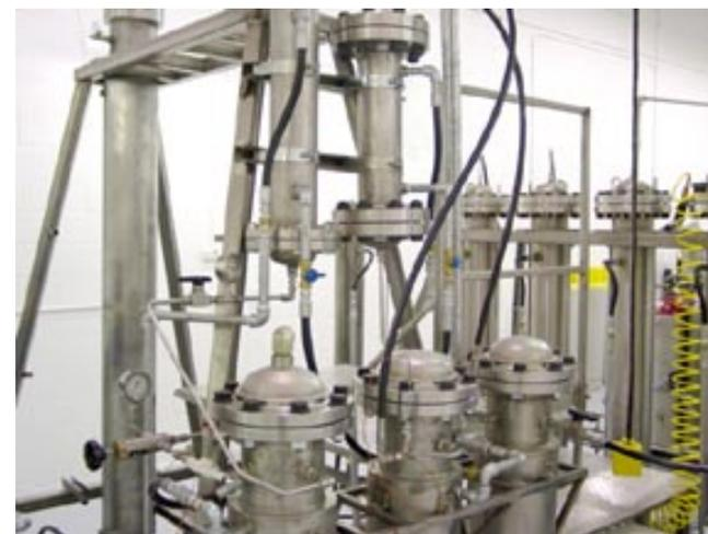
Pilot Plant Supercritical Fluid Extractor
