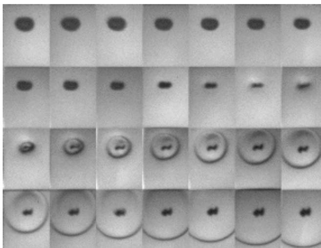
The series is taken with 20 million frames/s. The black area in the centre is the collapsing bubble and the circularly expanding halo starting in the third series is a shock wave.
