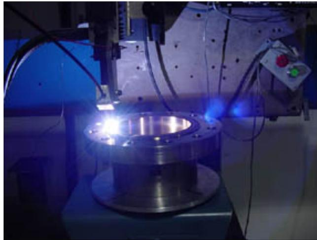
Automated Welding of Pressure Vessel
