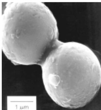
Two particles of zinc fused together after ultrasonication.
