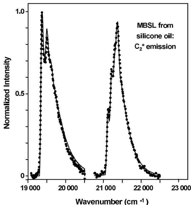
Figure 5. Excited-state  $C_2$  MBSL spectrum from silicone oil under Ar. Emission from the  $\Delta v = +1$  manifold of the  $d^3\Pi_g - a^3\Pi_u$  transition (Swan band) of  $C_2$  (Suslick *et al.* 1986). Observed MBSL spectrum from polydimethylsiloxane oil under Ar at  $0^\circ\text{C}$  ( $\cdots$ ). Best-fit synthetic spectrum for these two bands, with  $T_v = T_r = 4900\text{ K}$  (—).
