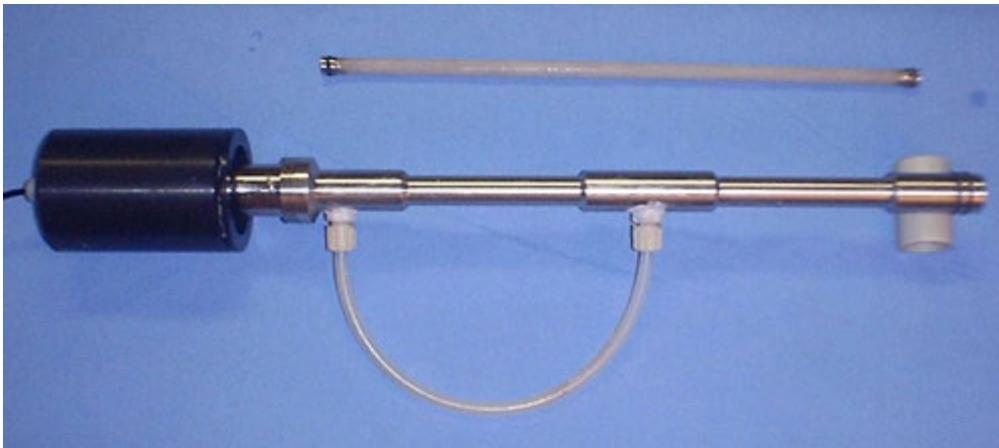
Example: Transducer mounted directly to filter housing end.
