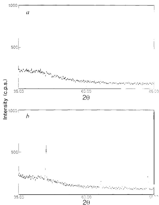
FIG. 3 X-ray diffracton powder patterns of amorphous iron powder (a) before heat treatment and (b) after crystallization at 350 °C for 6 h. Data collected on a Rigaku D-max diffractometer.
