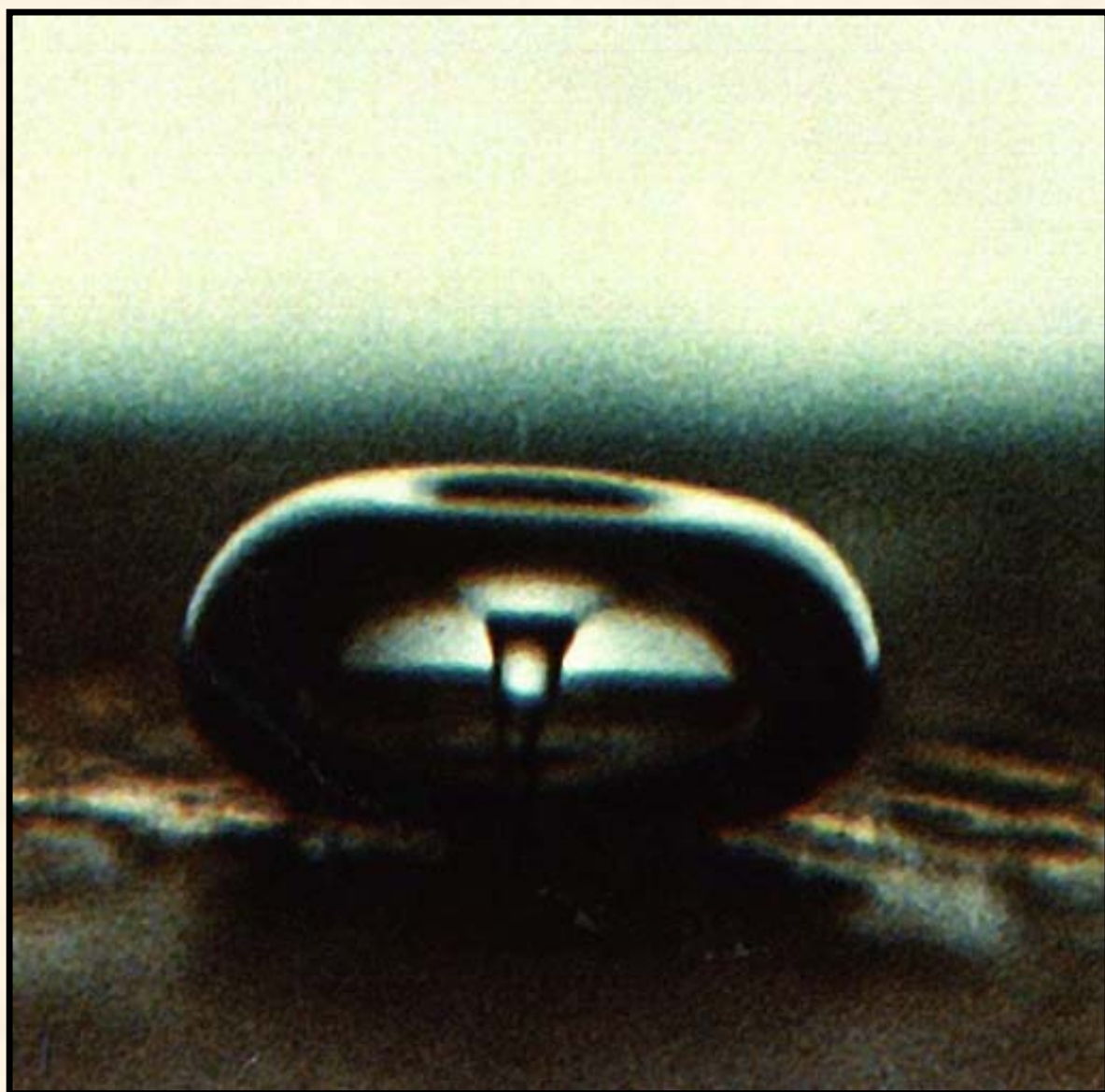
Figure 5. A bubble in a liquid irradiated with ultrasound implodes near a solid surface. The presence of the solid causes the implosion to be asymmetrical, forming a high-speed jet of liquid that impacts the surface. The cavity is spherical at first, but as it collapses the
