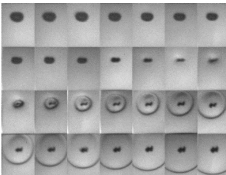
The series is taken with 20 million frames/s. The black area in the centre is the collapsing bubble and the circularily expanding halo starting in the third series is a shock wave.
