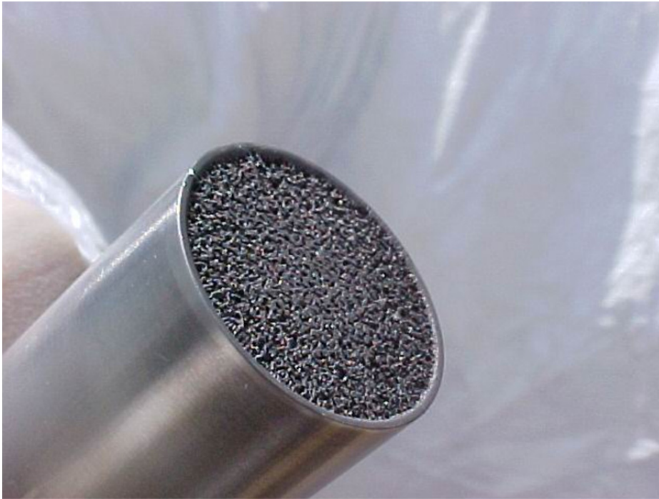
Erosion of sonotrode after 3 months of operation: 1000 watts, 20 kHz
