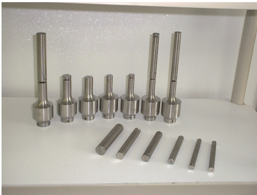
Erosion of sonotrode after 3 months of operation: 1000 watts, 20 kHz
