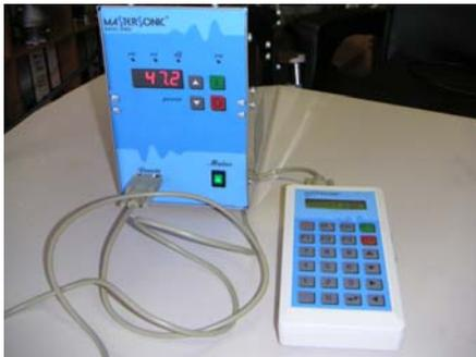
**Handheld controlled generator with MSH-1 controller unit**
