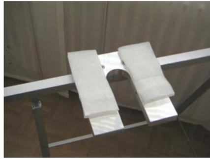
Reactor holder with foam-type backing placed in order to avoid direct metal-to-metal contact between the Clamp parts and the holder base-plate
