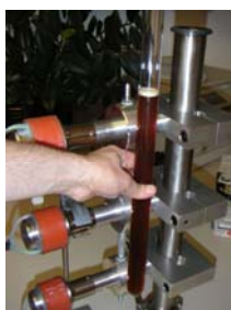
Glass tube can be fully submerged inside of the reactor
