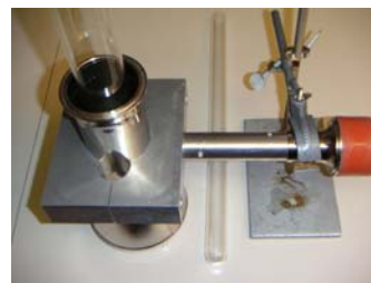
Water-coupling: temperature can be easily controlled
