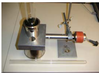
Glass tube inside of the MMM Reactor
