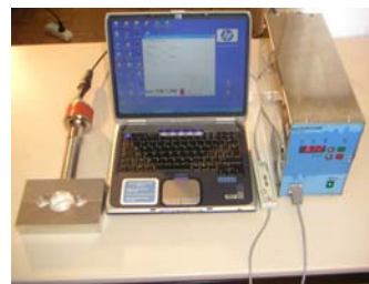
MMM generator and Clamps PC-controlled: all parameters programmable
