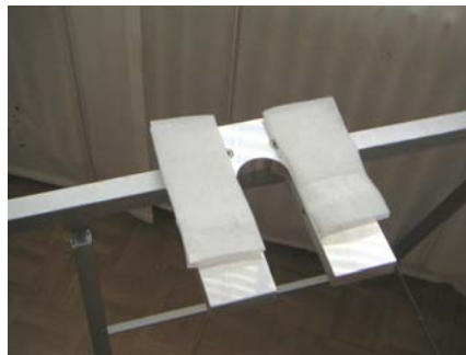
Reactor holder with foam-type backing placed in order to avoid direct metal-to-metal contact between the Clamp parts and the holder base-plate
