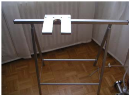
Reactor holder example, with the base-plate where the Reactor may hang.
