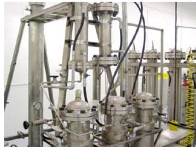
Pilot Plant Supercritical Fluid Extractor
