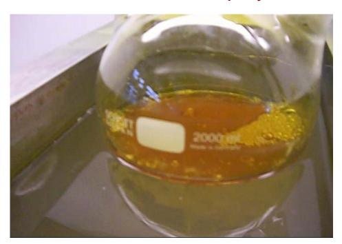
Minerals with precious metals content in glass vessel with acids mixture. MMM ultrasonic processing switched ON and OFF (see the difference in extracting activity)
