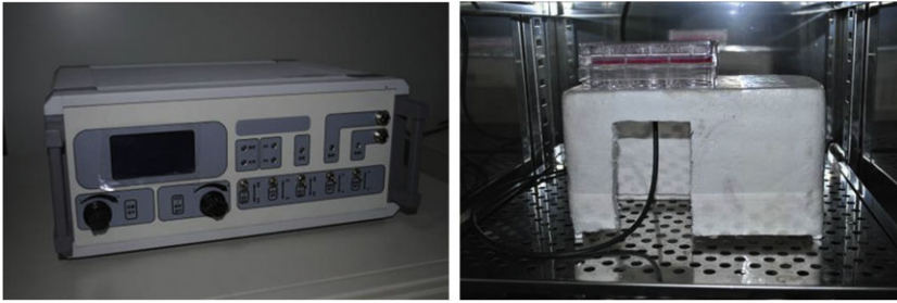
FIG. 1. US device for the application of pulsed US in vitro. The US device consists of a control box and an array of two transducers, each 30 mm in diameter specifically designed for a 6-well culture plate. Each channel could be individually tuned to give an output of 100, 150, and 200 mW/cm 2 . The culture plates were all placed in the incubator (37°C, 5% CO 2 , 95% humidity).
