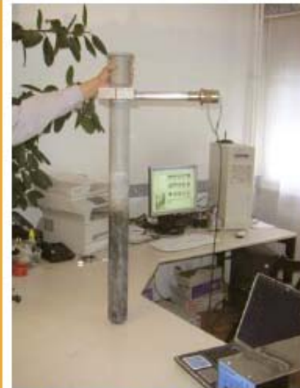
Clamp-On Ceramic tube for Liquid Metals Treatment
