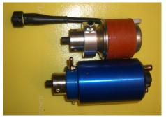
High power converters with air and/or water cooling
