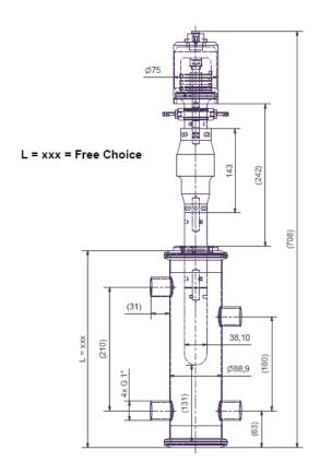
**Standard delivery set:** Ultrasonic Converter, Booster (only one), Flex-mount Resonator, Spherical Sonotrode, and Reactor Vessel-88 with flanges and fast clamps/covers.
