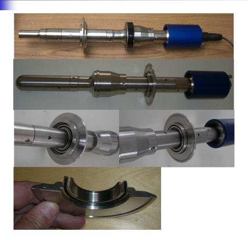
Converter - booster - flex-rigidmount - sonotrode: Good for low and moderate gain boosters
