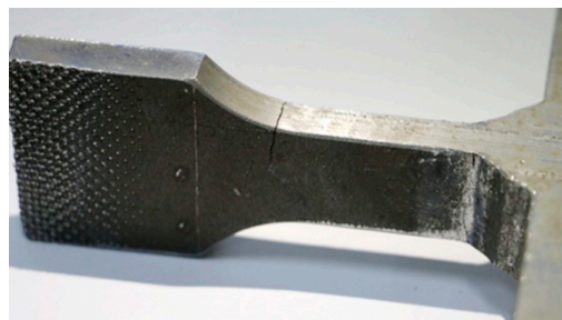
Figure 9. Fracture position of a welded joint of a sample that received UPT reapplications (Number of cycles: 1,104,878 cycles, delta sigma: 255 MPa).
