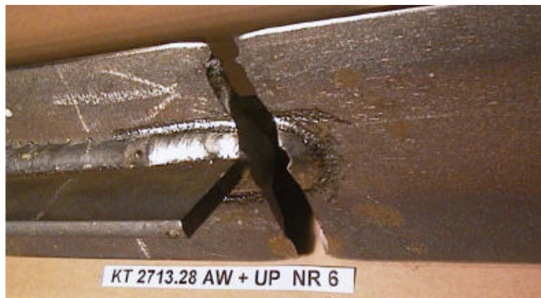
Fig. 6 Example of failure initiating at the root of the fillet weld in specimen treated by TIG dressing plus ultrasonic impact treatment.
