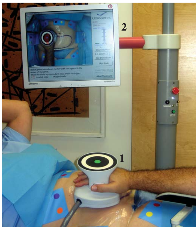
Fig. 1: System components: 1- the treatment transducer; 2- the user interface, showing the treatment area
